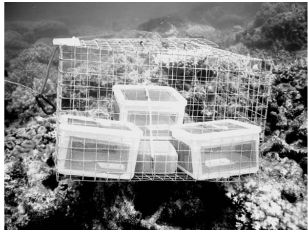
Fig. 2 Wire cage holding three feeding sub-cages, each with 1 mm mesh
